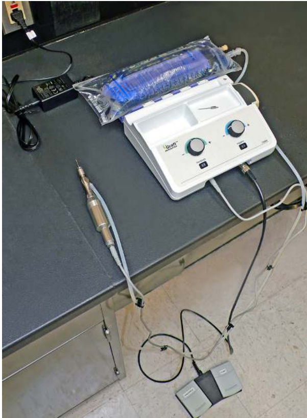
Fig. 2. Equipment set up showing irrigation system in place.
